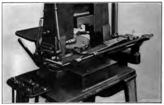
Fig. 10. Rear View of Dial Feed Operating Mechanism
